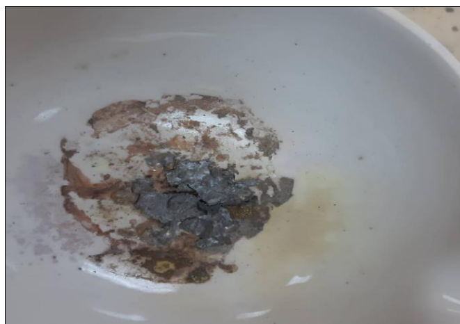
Figure 2. Precipitated silver recovered from used X-ray films via Sodium Hydroxide method
