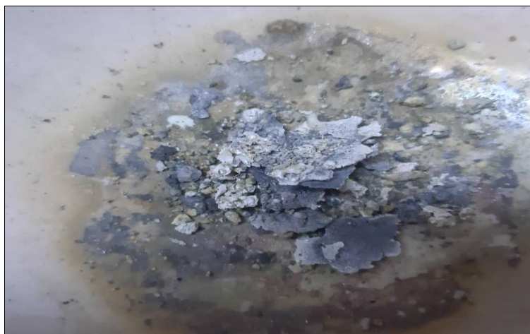
Figure 1. Precipitated silver recovered from used X-ray films via the Nitric Acid method
