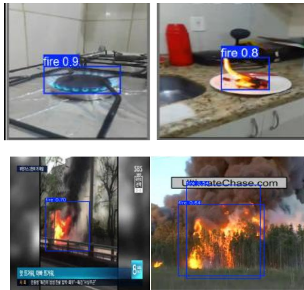
Figure 5. Sample testing results of the model for fire detection
